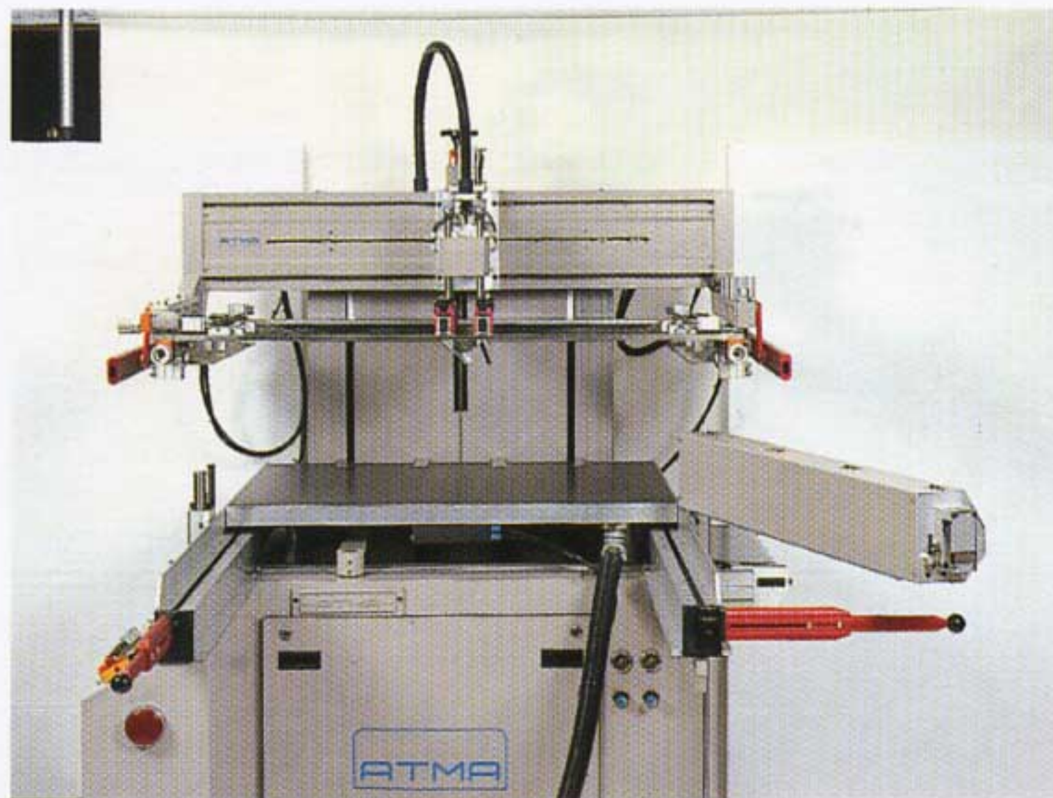
Open-front for easy setup & cleaning (Cleaning Roller is optional)
