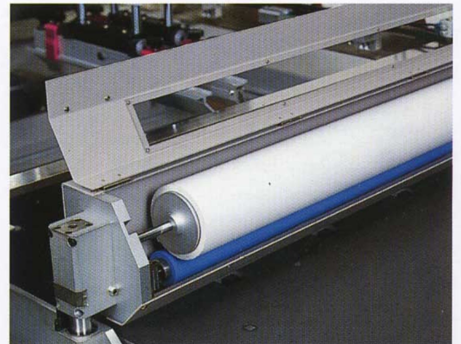
Cleaning Roller with Adhesive Tape (Optional, /R or /GR type)
