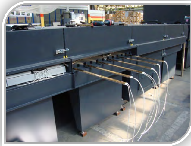
AirJet IR/QUARTZ TUBES EASY ACCESS
