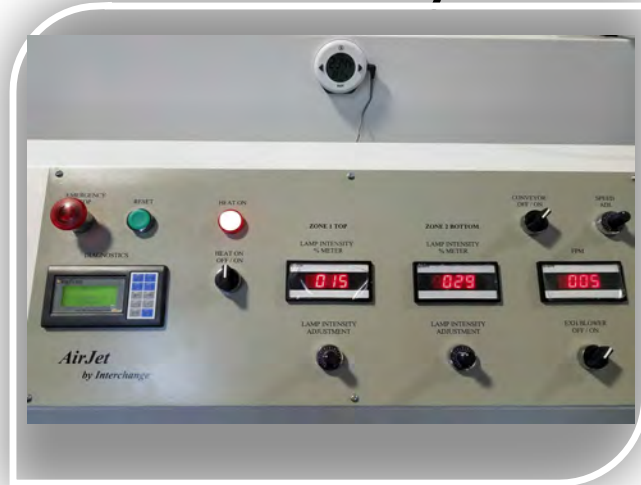
Solar Panel Curing Dryer - Percentage Display
