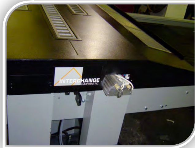
UVJet – SIDE MAGAZINE LOADING OF UV CASSETTE AND BULB CHANGE
