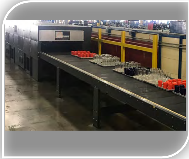
Extended Infeed with rigid support enables multiple printers feeding one dryer - Maximum Production
