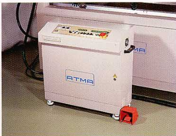
Mobile Electric Box
